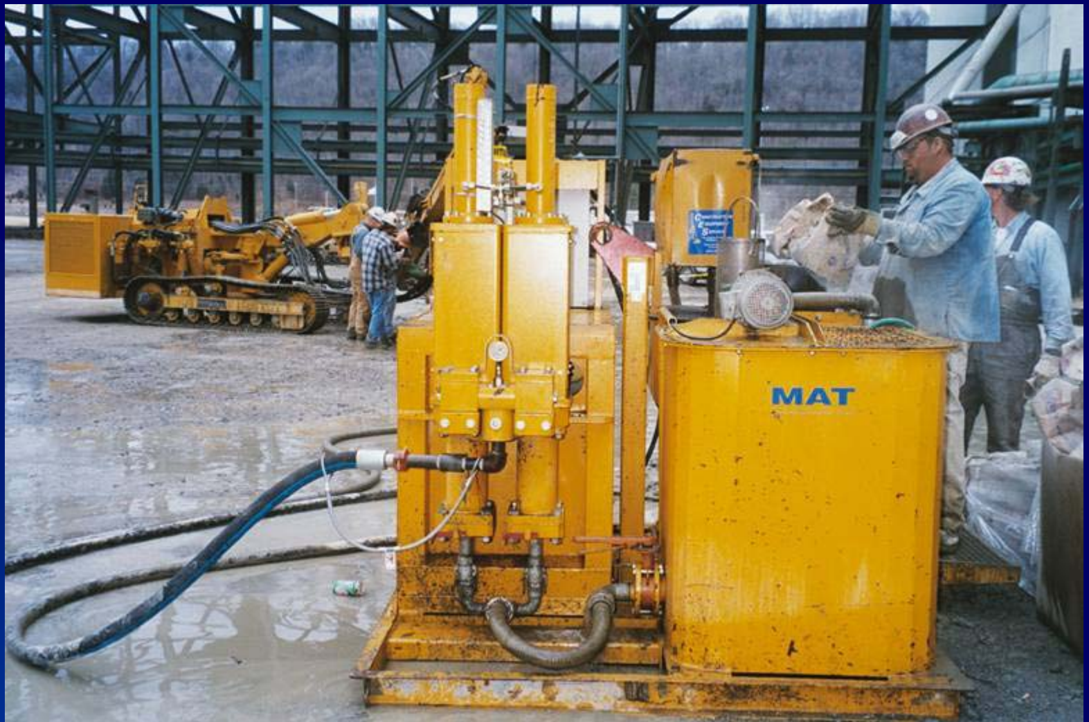
MAT mixer, one holding tank and double plunger pump
