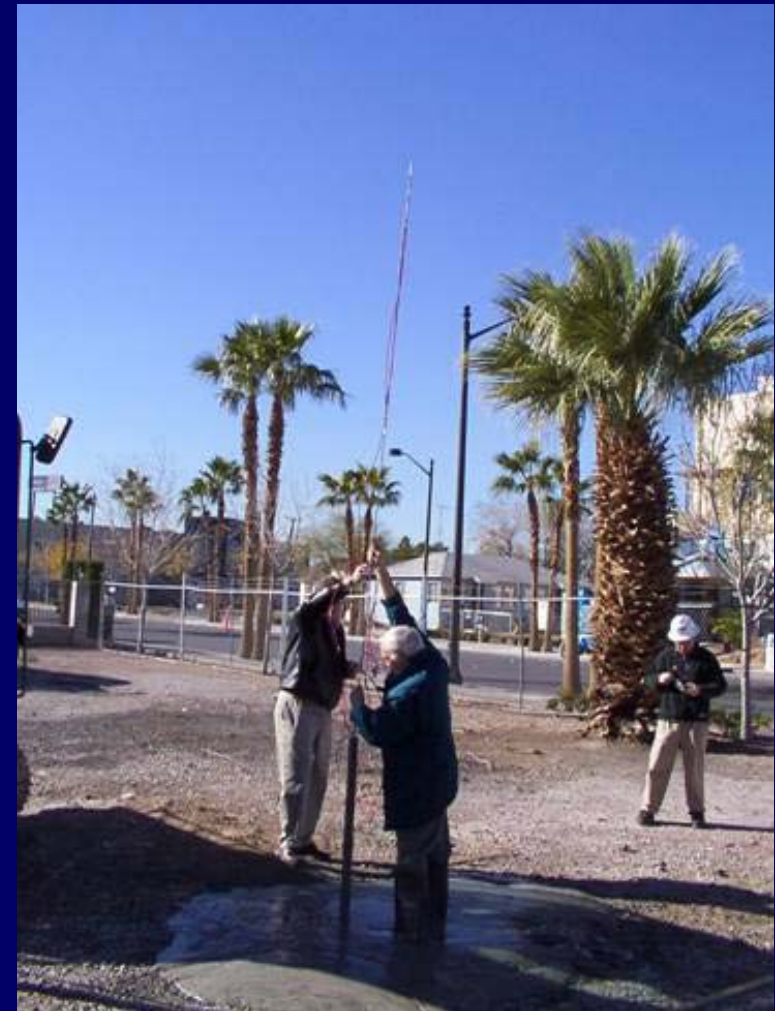
Installing strain gauges on a fiberglass rod pushed into a hollow bar
